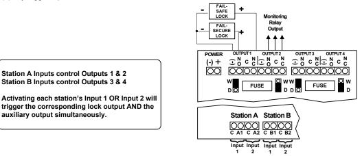
Each of the four outputs may be individually configured to operate as a conventional relay or a time delayed relay.
