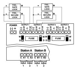
Each input may be individually configured to operate as a conventional relay or a time delayed relay. Alternatively, each input may be individually configured to operate as a latching relay or a time delayed relay.
